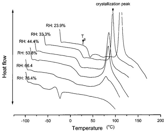
**Figure 4.** DSC thermal curves for amorphous lactose/sucrose/invertase samples, after equilibration at different water activities (24 °C).
