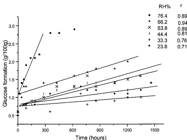
**Figure 6.** Example of first-order plots of sucrose hydrolysis.
